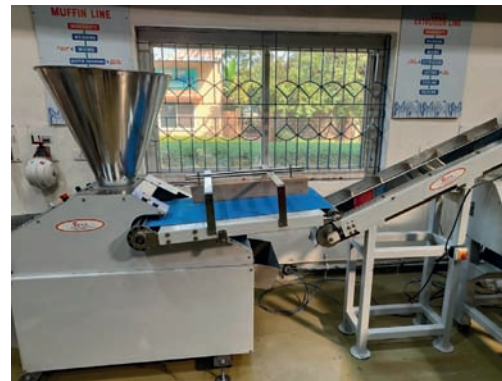
Figure 2.40 Conical Dough Divider Machine
