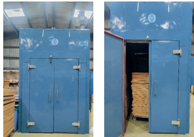
Figure 2.36 Static Tray Drier
