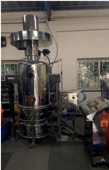
Figure 2.69 Fluidized Bed Dryer
