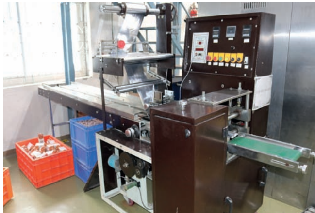
Figure 2.28 Tray Packing Machine
