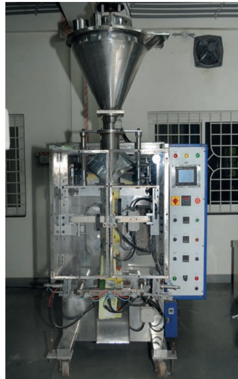
Figure 2.60 Vertical Form Fill Packing Machine
