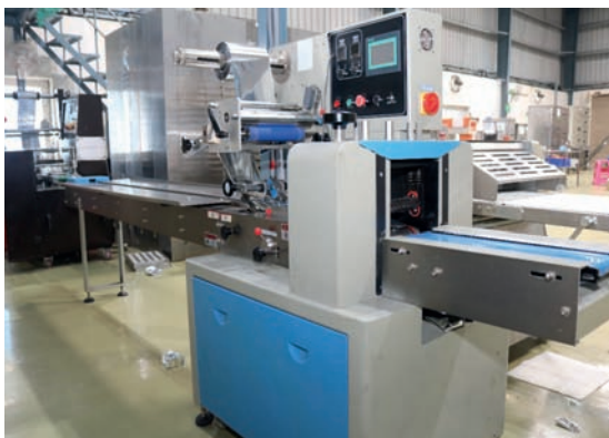
Figure 2.32 Horizontal Flow Wrap Machine
