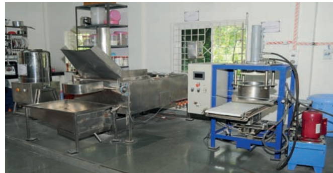
Figure 2.67 Murukku Machine and Deep Fryer
