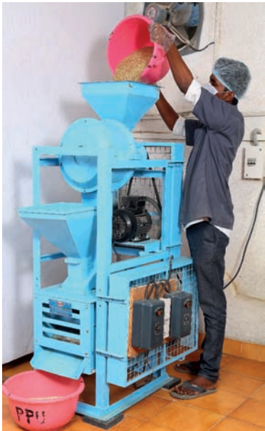
Figure 2.15 Dehuller cum Separator
