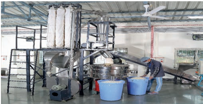
Figure 2.63 Jowar Grinding Plant
