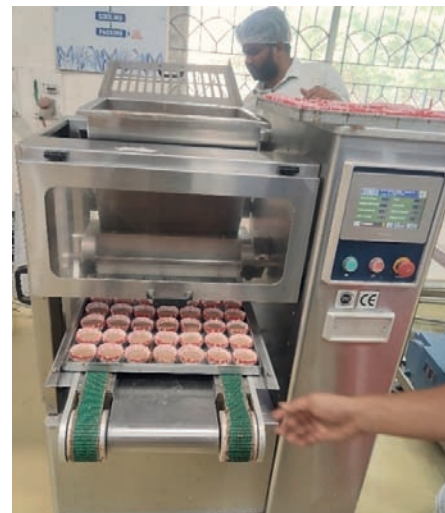
Figure 2.33 Muffin Dropping Machine
