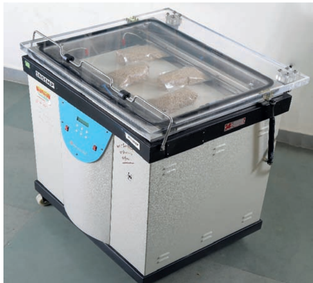
Figure 2.61 Vacuum Packing Machine
